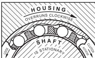
Clearance between the rollers and cup ramps is exaggerated in these drawings.
