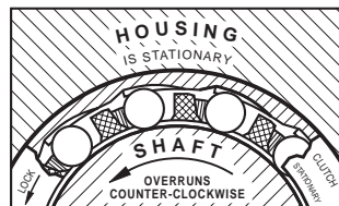
Clearance between the rollers and cup ramps is exaggerated in these drawings.
